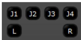
Buttons J1–J4, L, and R are Joystick key emulations. They can be configured accordingly in the workstation's configuration file (see Administrator's Guide).
