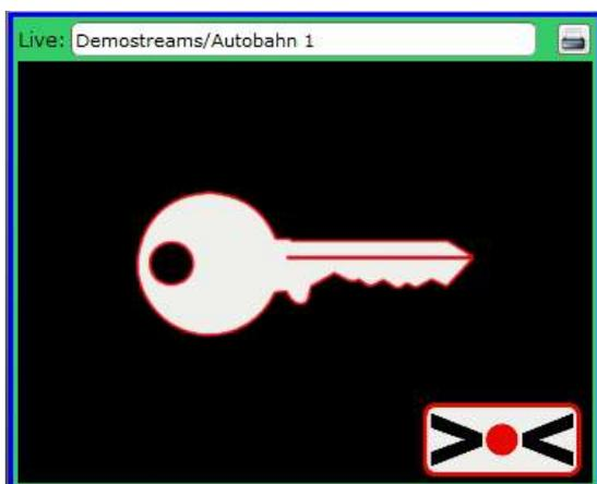
Figure 3-24: View of encrypted camera streams without connected dongle
