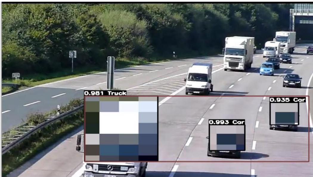
**Figure 3-41: Object detection wit displayed confidence value and activated pixelation**
